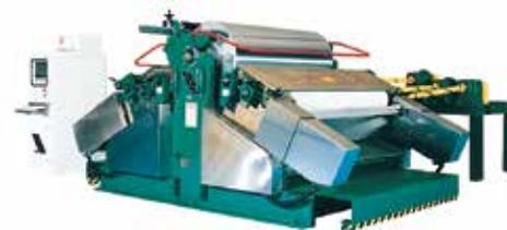
**LAMINATOR/EMBOSSER:** Normally located at the finish oven exit, GFG Laminators apply a variety of films or emboss a previously coated strip. Supplied with this system are the guides, controls, unwinds, edge trim unit and scrap removal system.
