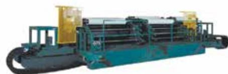
**DUAL-HEAD FINISH COATER:** The "dual-head" design of this GFG Finish Coater provides an economical solution for quick color changes on the topside coating. While disengaging one topside head, the second topside head is engaged allowing for extremely efficient color changes with a minimal amount of scrap being generated. The Dual Topside Coater provides a quick color change solution for your line when space constraints prevent the use of other coater configurations.
