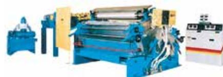
**QUICK COLOR CHANGE SHUTTLE COATER:** This Shuttle Coater was designed to improve your production capabilities by enabling color changes in approximately 30 seconds. While coater operators cleanup one set of coating rolls and pans, another set of rolls is in operation eliminating costly downtime. Shuttle Coaters can be equipped with two sets of topside heads, two sets of bottomside heads, or dual heads on both the topside and bottomside.
