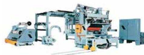
**VERTICAL WAXER:** The GFG Vertical Wax Coater is designed to melt and apply a thin film of lubricating wax to the strip for products such as can end stock.
